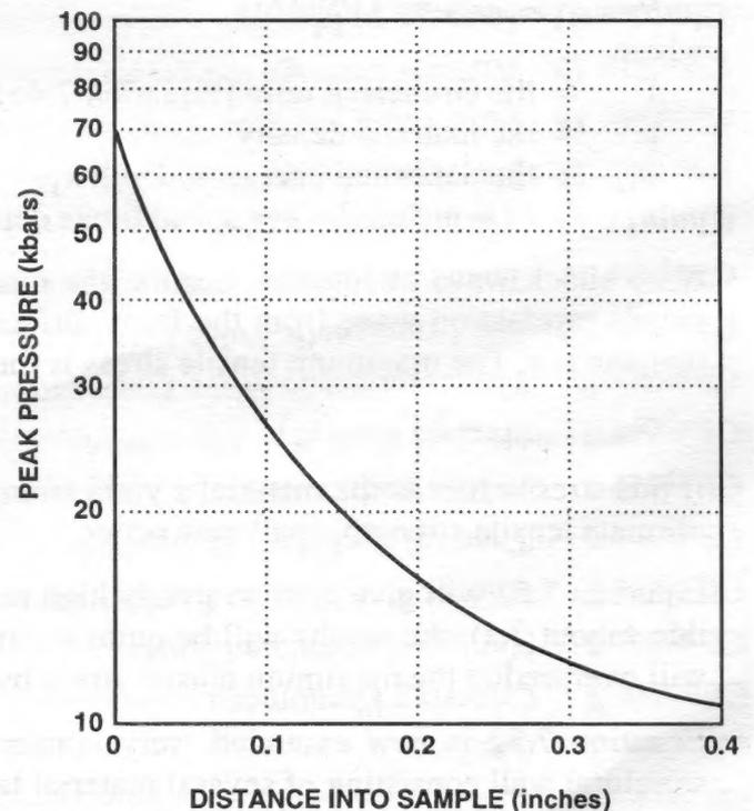
Figure 7.12. Shock Attenuation in Tape-Wound Silica Phenolic for a 10-ktap Pulse.
